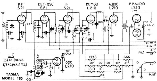
Tasma model "150" is an 8-valve receiver designed to provide broadcast coverage and operation from battery power supply. This receiver is of the console type and is fitted with three controls, these being for volume, tuning and battery-switching (2-circuit). This receiver uses an 8-inch diameter permag. loudspeaker with a 10,000 ohms plate-to-plate transformer and was marketed
